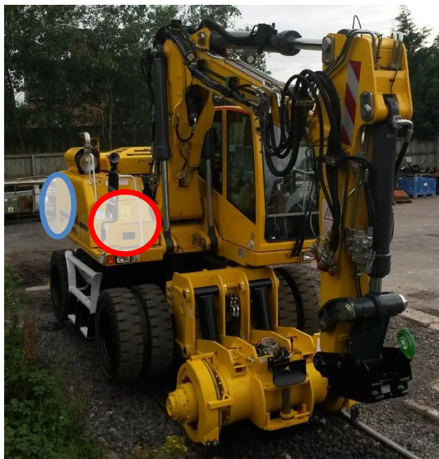
Figure 3 - Engine and Hydraulic Bays - Over-ride Key Locations
