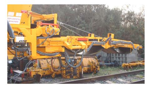
WITH THE CONVEYOR IN ITS FULLY DEPLOYED POSITION PULL DOWN ON THE "TENSION BELT" LEVER.
