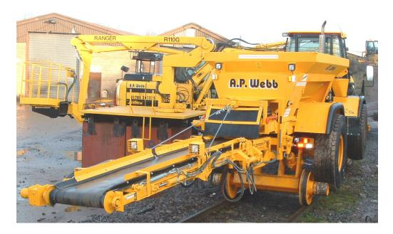
THE CONVEYOR CAN NOW BE RUN FROM INSIDE OR OUTSIDE OF THE CAB.
