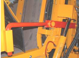
• WITH THE SUPERBOSS' ENGINE RUNNING SWITCH ON THE "PP" IN THE CAB. SWITCHING THIS TO ITS MIDDLE POSITION ACTIVATES THE BALLAST UNLOADER SYSTEMS. SWITCHING IT AGAIN OPERATES THE WORKING LIGHTS.
