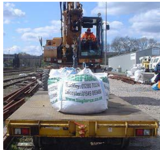
Figure 10 Loading sequence for a partial load
