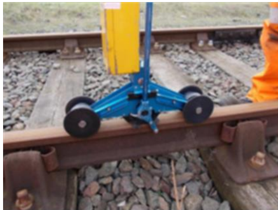
Figure 2 – Pre use check of a trolley without rail wheel braking
