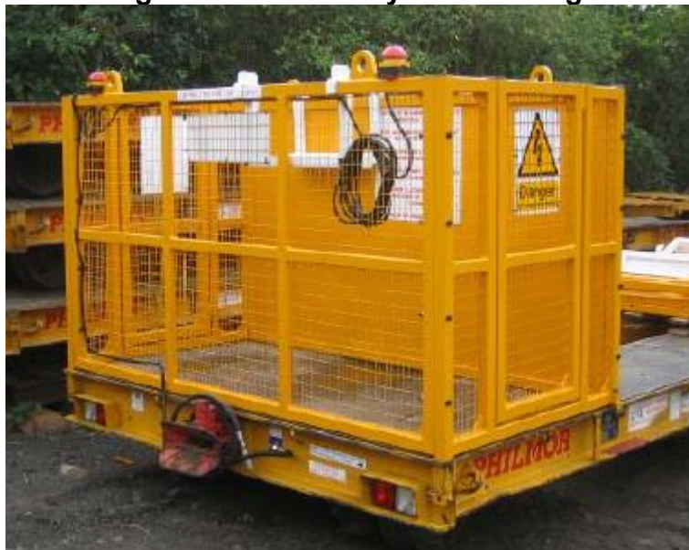
Figure 7 – Correctly secured cage
