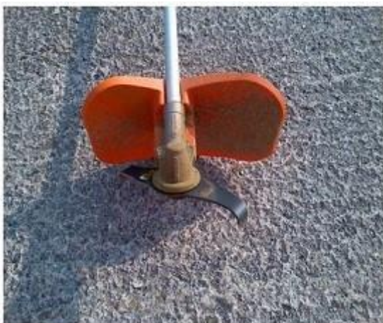
Figure 1: Brush cutter with shredder blade and correct protective guard fitted
