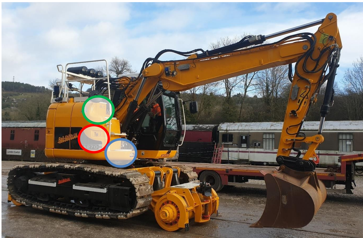
Figure 5 - Engine and Hydraulic Bays - Over-ride Key Locations
